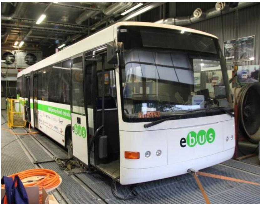
*Test Mule being tested with VTT's heavy vehicle dynamometer*
